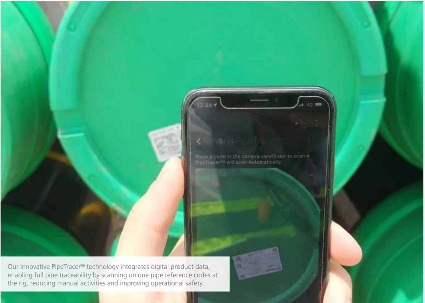
Our innovative PipeTracer® technology integrates digital product data, enabling full pipe traceability by scanning unique pipe reference codes at the rig, reducing manual activities and improving operational safety.
